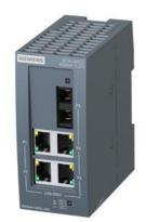
SCALANCE XB004-1LDG unmanaged Industrial Ethernet Switch for 10/100/1000 Mbit/s; for setting up small star and line topologies; LED diagnostics, IP20, 24 V DC power supply, with 4x 10/100/1000 Mbit/s RJ45 Ports electrical and 1 x 1000 Mbit/s SC port optical (single-mode, glass), up to max. 10 km Manual available as a download
